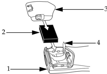
**Figure 7: Inserting Battery into the SDR 8100**
