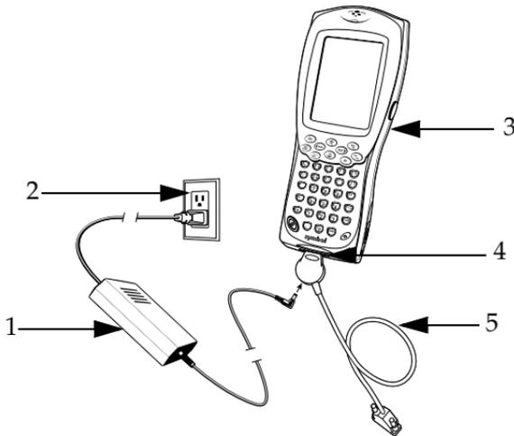
**Figure 8: Charge Battery Using Synchronization Cable**
