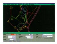
SDRmap is the base module of the SDR Mapping and Design system. It is the complete field data processing module giving you automatic reduction of raw data to coordinates and automated mapping from sophisticated analysis of feature codes entered during data collection. Literally, the push of a button takes you from raw data to finished hard copy plan. Data reduction features include:
