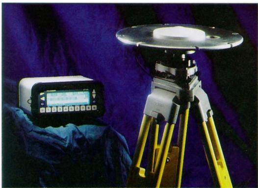
**Sokkia's GSR2100 provides high-precision GPS measurement, and is upgradeable to real-time kinematic capability.**
