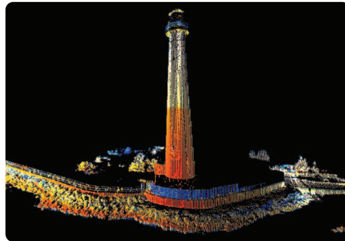
Lighthouse Dynascan Point Cloud from open sea
