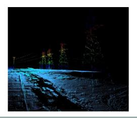
Throughout the project the Dynascan continued operating and collecting data. A vast amount of data was produced, cleaned and adjusted. The finalised point clouds produced matched up perfectly with the data collected from the survey boats and offered great value to the project contractors.
