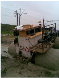
An RTK base station at the centre of the project area provided GPS corrections, picked up by the Dynascan's radio antenna. System checks were done twice a day, when the buggy was driven past areas that had been densely surveyed by conventional means. Each night, the scanned data would be compared with the surveyed data for a confidence check on the absolute position of the survey and the quality of the scanning laser pitch, roll and heading sensors in the Dynascan.
