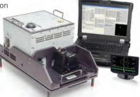
Its unrivaled small size and lightweight configuration give the Orion-C exceptional flexibility—quick to install in any type of aerial vehicle, including helicopters, fixed-wing aircraft and even UAV platforms. Fast-mounting, with minimal cabling and easy to transport, the Orion-C delivers optimized and cost-effective data collection missions.
