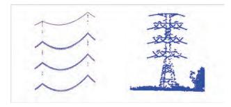
Power line and tower point cloud output from ALTM Orion-C data. Data set reveals complete top wire detection, wire separation within a 4-wire bundle, and detailed tower architecture delineation for easy tower type detection.
