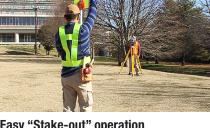
Stake-out can be easily done by automatic turning and guide light.
