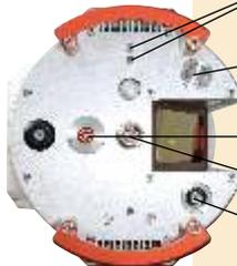
Mounting points (3x) and mounting threads inserts (2x) for digital camera
