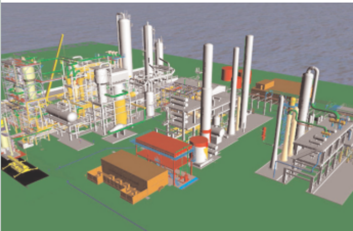
Factory site as 3D model – generated from scanner data
