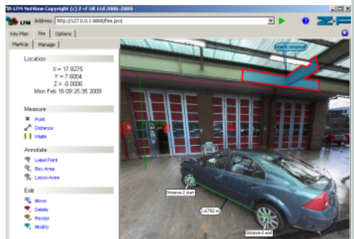
Measurements and mark ups in LFM NetView
