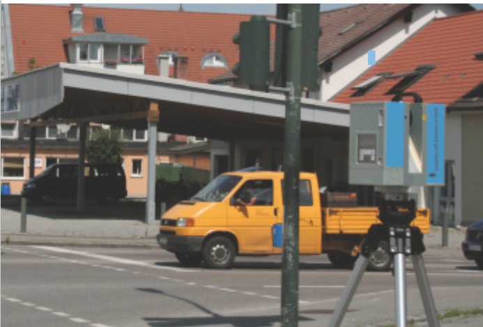
Laserscanning in infrastructure facility
