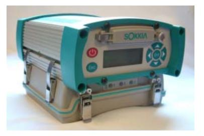
The GSR2600 is a high-performance GPS receiver for use in both RTK and post-processing applications. This receiver is capable of **receiving and tracking up to 12 GPS satellites** on L1 and L2 channels, has **fast data update rates**, and **integrated memory** (Compact Flash Card) for data logging.
