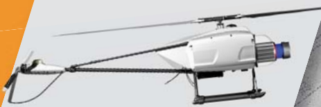
VUX ® -1 mounted on UAS, e.g. Flying-Cam 3.0 SARAH
