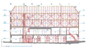
TachyCAD enables transmission of measurement data from a total station to a notebook. At measurement initiation, the data is automatically transferred to the notebook. TachyCAD calculates and plots the 3D coordinates of the point. The survey data is made available for AutoCAD drawing and design processes in the same way as pointing with a mouse or
