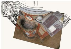
On the basis of a few measured control points PhoToPlan Pro and PhoToPlan Ultimate calculate the camera position, direction and distortion of the images.
