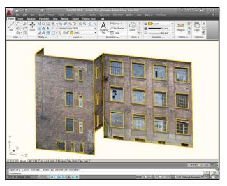
With PhoToPlan you may rectify photos for a 2D evaluation either with a few reference lengths from the object or with control points which have been measured on the object. The rectification planes may be positioned freely.
