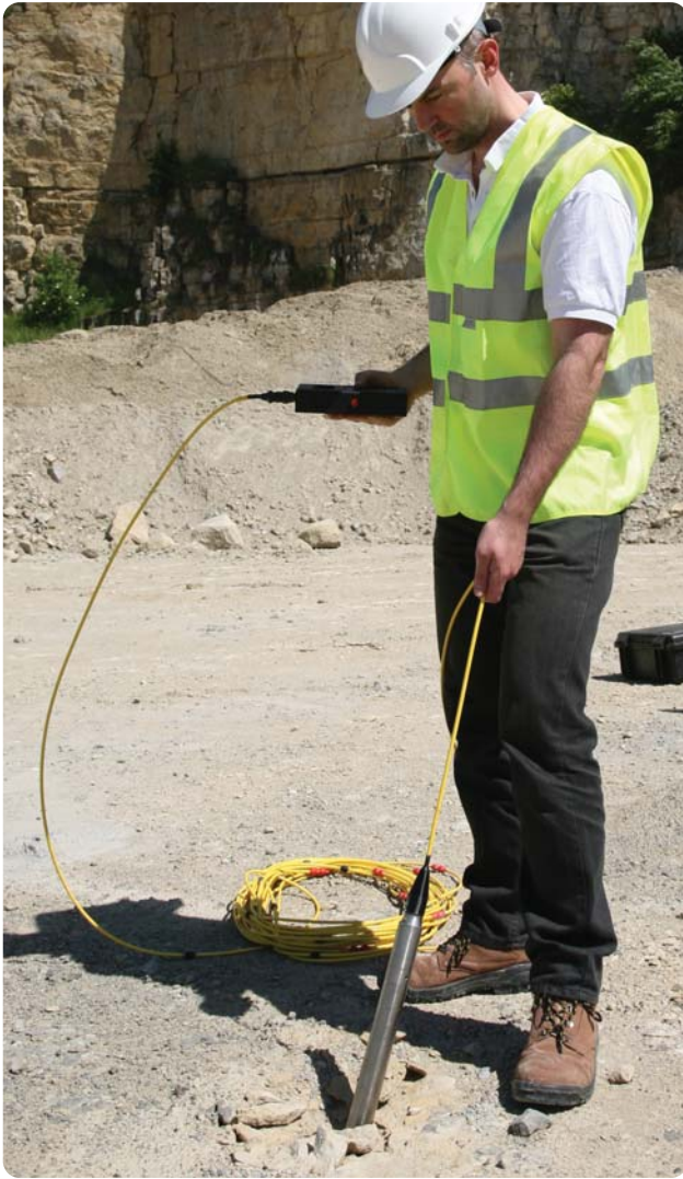
Cabled Boretrak® showing complete system including CDU logger
