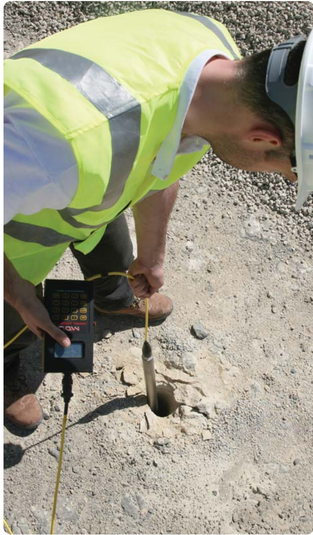
Cabled Boretrak® being lowered by hand into borehole
