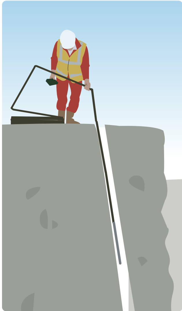
Rodded Boretrak ® being lowered down borehole
