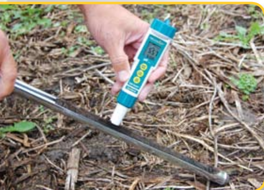
SoilStik shown in use with Item 6510, Model HC Soil Sampler (page 51)
